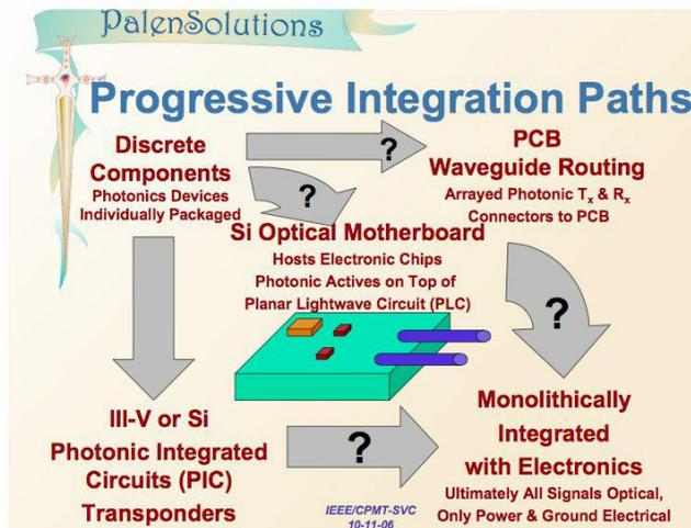
Fig. 2. Integration pathways from discretely packaged photonic components to photonic circuits monolithically integrated with electronics<sup>5</sup>.
