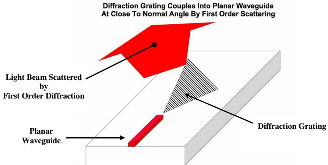
Fig. 4. Diffraction gating coupling to photonic chip.
