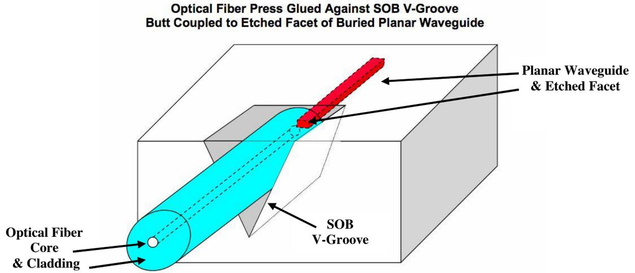
Fig. 3. Butt coupling of optical fiber in SOB v-groove to PLC waveguide.
